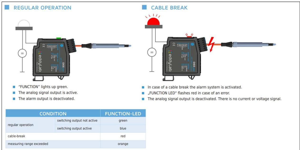
It may be necessary to reduce the sensitivity of the cable break detection if there is a high EMC load. Under certain circumstances, external faults can trigger an unintentional false alarm. This can also occur when operating third-party devices on the DEEneo. In such cases, adjust the "Alarm Threshold" value. If desired, you can also completely deactivate cable break monitoring. To do this, set the "Enable Alarm" field to False.
