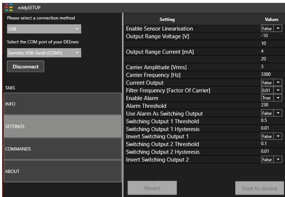
The menu is divided into 4 tabs in the left-hand column: About, Info, Settings and Commands. In the right-hand column, the settings and information associated with the respective tab are displayed.
