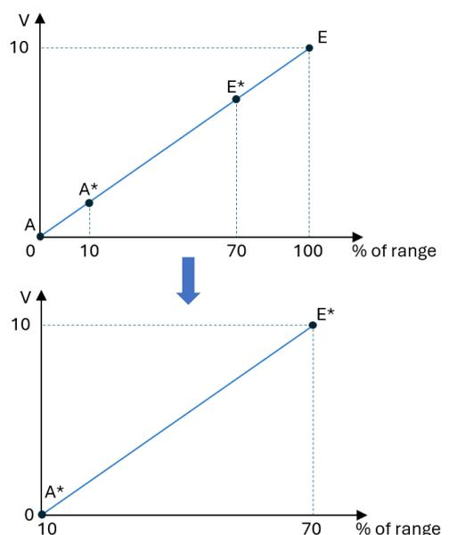
In the illustrations on the right, the output signal is scaled from 0...10 V to a reduced measuring range of 10...70 % of the nominal sensor measuring range (0...100 %).
